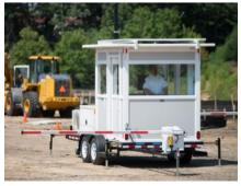
Adding video surveillance and lighting capabilities makes this a multi-purpose platform for many different applications. Ideal for construction, utilities, oil and gas and any other temporary work or storage areas requiring additional security.
